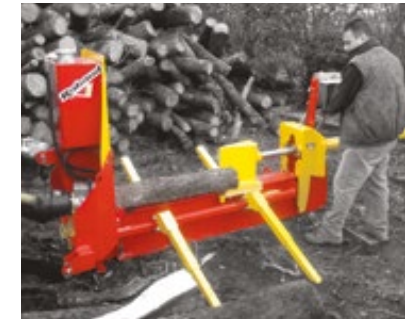
Log splitting with 1.15m clearance
