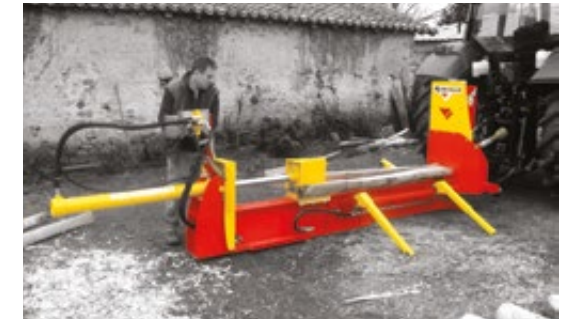
POLYCOMPACT post splitter: post splitting with max. clearance 2.25 m
