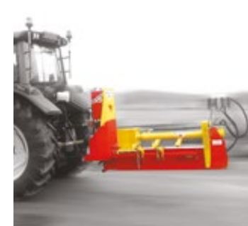
POLYCOMPACT post splitter, transported: 2.37 m
