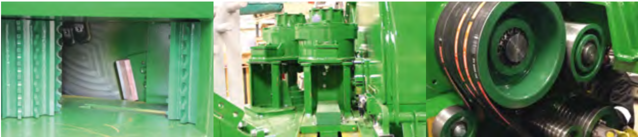
Split blades and cuts minimise wear on blades and optimises fuel economy.
