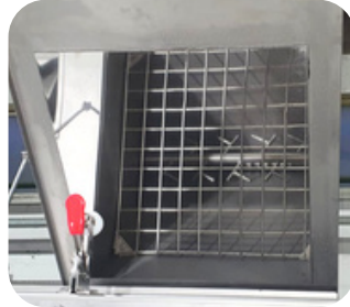
Detalle interior tolva y sinfín Interior detail of the hopper and the endless screw
