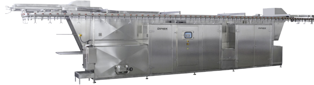
lavado aéreo de cajas y bandejas overhead washing of crates and trays
