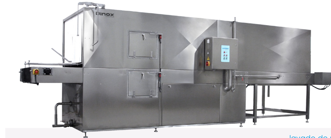
lavado de palots y cajas washing of palots and crates
