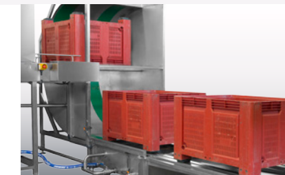
lavado de palots y cajas washing of palots and crates
