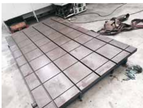
Mesa ranurada Dimensiones: 3500x2000x390mm Slotted table Dimensions: 3500x2000x390mm.
