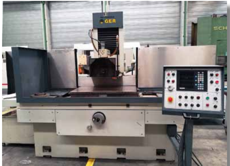
GER S-100/50. CNC FAGOR. Mesa: 1000x600mm. Muela: Ø 400x100x127mm. Plato magnético de polo fino: 1000x600mm. GER S-100/50. CNC FAGOR. Table: 1000x600mm. Grinding wheel: Ø 400x100x127mm. Fine pole magnetic chuck: 1000x600mm.
