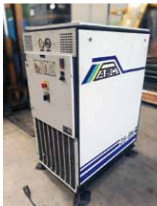
Compresor de tornillo ABC 25-BN ABC 25-BN screw compressor
