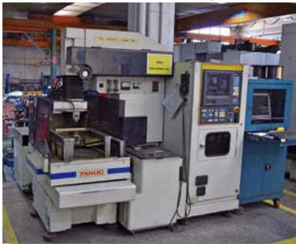
FANUC TAPE CUT W1. Recorridos: 350x250x250mm FANUC TAPE CUT W1. Travels: 350x250x250mm
