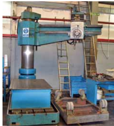
Taladro radial FORADIA MT-2000. Broca Ø: 75mm. Bandera: 2000mm FORADIA MT-2000 radial drill. Drill bit diam. 75mm. Arm: 2000mm
