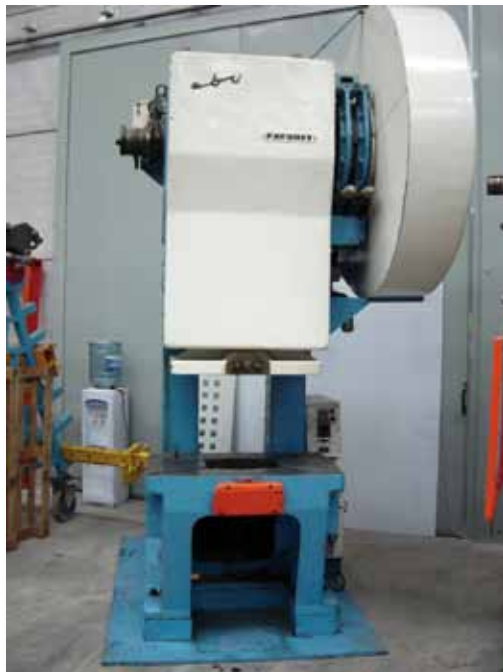
Prensa excéntrica GROTZINGER 100 Tn. Mesa: 900x600mm. 105 g.p.m. GROTZINGER eccentric press 100 Tn Table: 900x600mm. 105 s.p.m.
