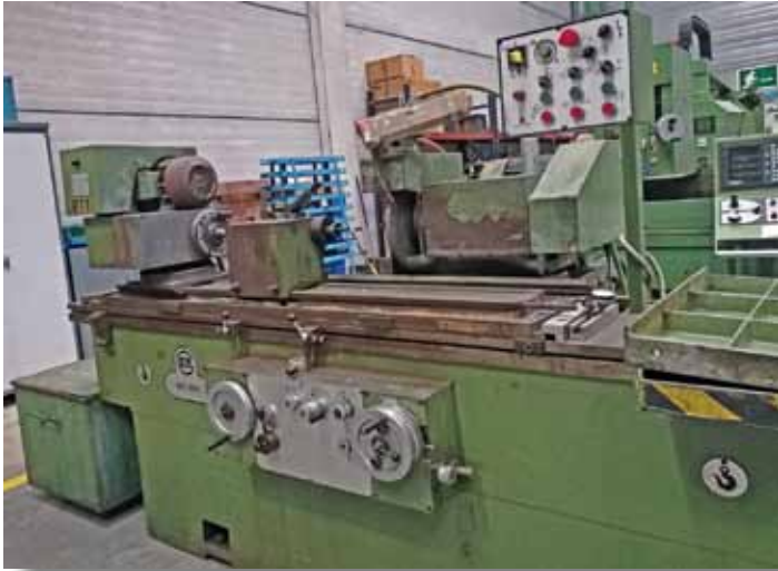
Universal GER RHC 1000 . Distancia entre puntos: 1.000mm Ø máx a rectificar: 355mm. Muela: Ø 400x50x127mm. Universal GER RHC 1000 . Distance between centers: 1,000mm Max grinding diam: 355mm. Grinding wheel: Ø 400x50x127mm.
