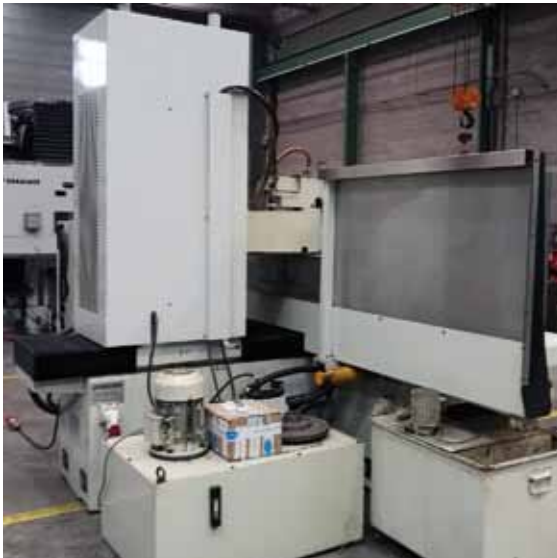
GER S-100/50. CNC FAGOR. Mesa: 1000x600mm. Muela: Ø 400x100x127mm. Plato magnético de polo fino: 1000x600mm. GER S-100/50. CNC FAGOR. Table: 1000x600mm. Grinding wheel: Ø 400x100x127mm. Fine pole magnetic chuck: 1000x600mm.
