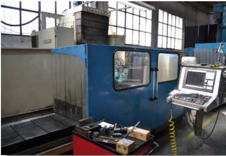
ANAYAK VH-2200. CNC FAGOR 8050 M. Mesa: 2200x600 mm. Recorridos: 2000x900x800mm. ANAYAK VH-2200. CNC FAGOR 8050 M. Table: 2200x600 mm. Travels: 2000x900x800mm.
