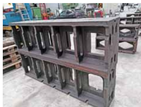
Mesa ranurada Dimensiones: 3500x2000x390mm Slotted table Dimensions: 3500x2000x390mm.
