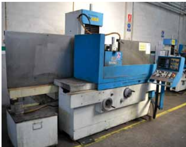
GER S-100/50. CNC FAGOR. Recorridos: 1160x500mm Muela: Ø 400x100x127mm. Plato magnético de polo fino: 1000x500mm. GER S-100/50. CNC FAGOR. Travels: 1160x500mm. Grinding wheel: Ø 400x100x127mm. Fine pole magnetic chuck: 1000x500mm.
