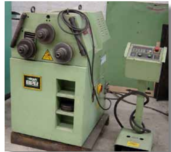
Curvadora de perfiles BPR CPS-35 . Ø ejes: 35mm. 3 rodillos. BPR CPS-35 profile bender. Axes Ø: 35mm Semi-new. 3 rolls.
