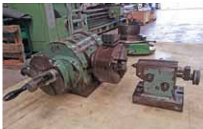
Platos divisores: Ø 140 – 160mm Rotary tables: Ø 140 – 160mm
