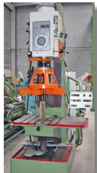
Taladro columna IBA TMA-75 Mesa móvil: 1100x800mm IBA TMA-75 Mobile column drill Mobile table: 1100x800mm
