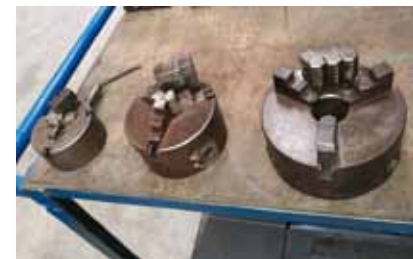
Platos torno: Ø 155-310mm Chucks: Ø 155-310mm
