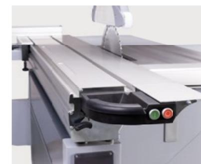
**Remote ON switch on sliding table**
