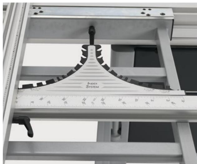
**Angle adjustment and fence length compensation**
