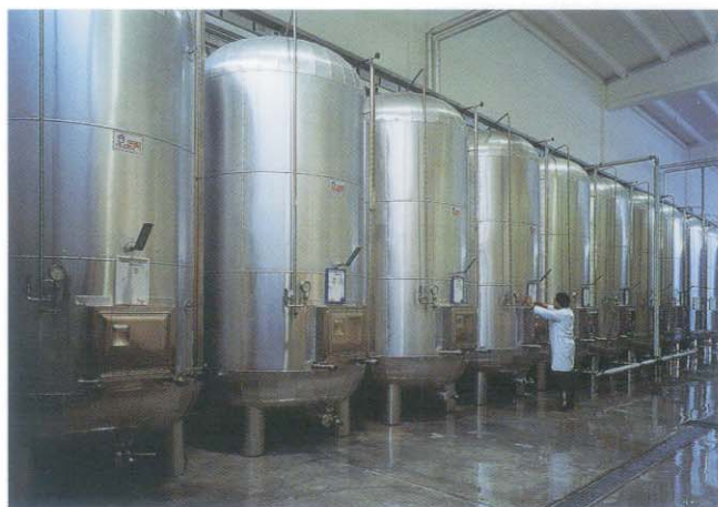
TOSO Pietro - Cossano Belbo (CN) - Autoclavi coibentate in acciaio inox. TOSO Pietro - Cossano Belbo (CUNEO) - Insulated stainless steel pressure tanks.
