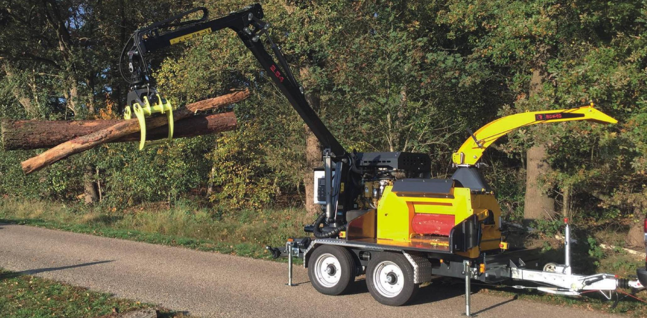
HASTA 70 M<sup>3</sup>/H HASTA 200 CV TRONCOS HASTA Ø400 MM
