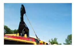
**OPTIONAL WINCH.** Eliminates the need to drag large material to the chipper. The 150' (45.7 m) winch line can handle material up to 4000 lb (1814.9 kg), making it easy to lift logs directly onto the feed table. In addition the winch can also be hydraulically raised out of the way to allow operators to feed the unit using a loader. Vermeer
