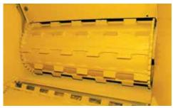
LOWER FEED ROLLER. The lower feed roller is offset from the upper feed roller by 10.8" (27.4 cm). Material is easily pulled to the upper feed roller, so there is less need to manually raise the upper feed roller for larger diameter material.
