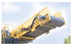
**DISCHARGE CONVEYOR.** Create a spacesaving continuous stack or a 20' (6.1 m) wide by 9' (2.7 m) high windrow configuration depending on site needs and space considerations.
