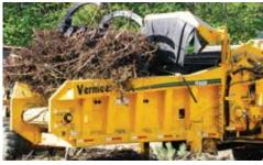
PROGRESSIVE PROCESSING. The patented SmartGrind system monitors engine rpm and adjusts grinding speed to increase productivity. The open-ended, wide infeed table makes material loading easy and efficient.
