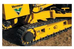
**ZERO TURNING RADIUS.** The planetary traction drive helps provide increased traction while the counter rotating tracks provide tight maneuvering in difficult jobsite conditions.
