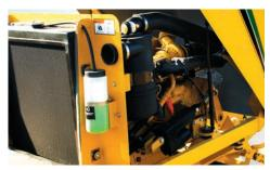
**POWERFUL PERFORMANCE.** With its 60 hp (45 kW) diesel liquid-cooled engine, the SC60TX packs the power needed for bold performance.
