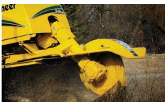
PATENTED GEARBOX DRIVEN CUTTER WHEEL SYSTEM. This system directs the maximum amount of horsepower to the cutter wheel and it is a more efficient drive as compared to other systems on the market. There is no side load on engine and unlike a belt drive, there are no belts to adjust or align.
