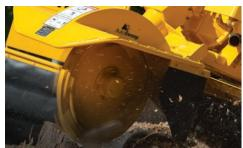
**AUTOSWEEP.** The patented AutoSweep® system monitors engine speed and automatically adjusts cutterwheel sweep rate to maximize power to the cutter wheel while reducing engine stress.
