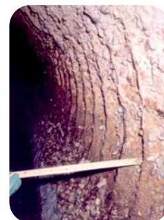
Effects of external and internal corrosion on pipes
