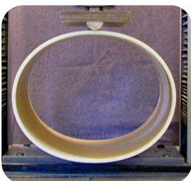
The flexibility of plastic pipes is important to absorb ground movements
