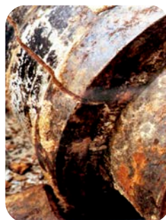
Effects of external and internal corrosion on pipes
