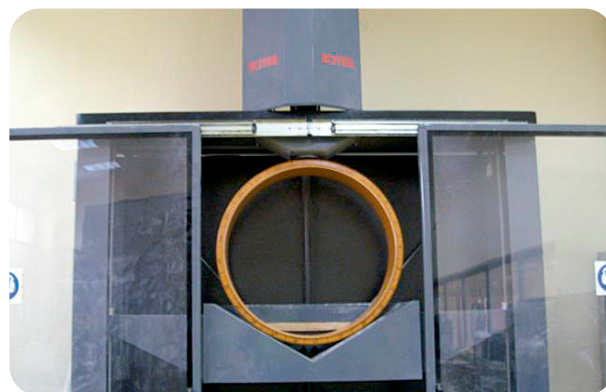
Stiffness testing of a flexible pipe
