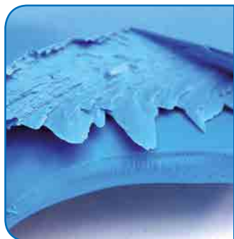
When PVC with its amorphous structure (lower section) is subjected to the orientation process, a laminate structure is obtained (upper section).
