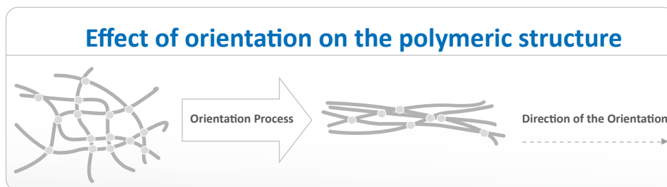
When PVC with its amorphous structure (lower section) is subjected to the orientation process, a laminate structure is obtained (upper section).
