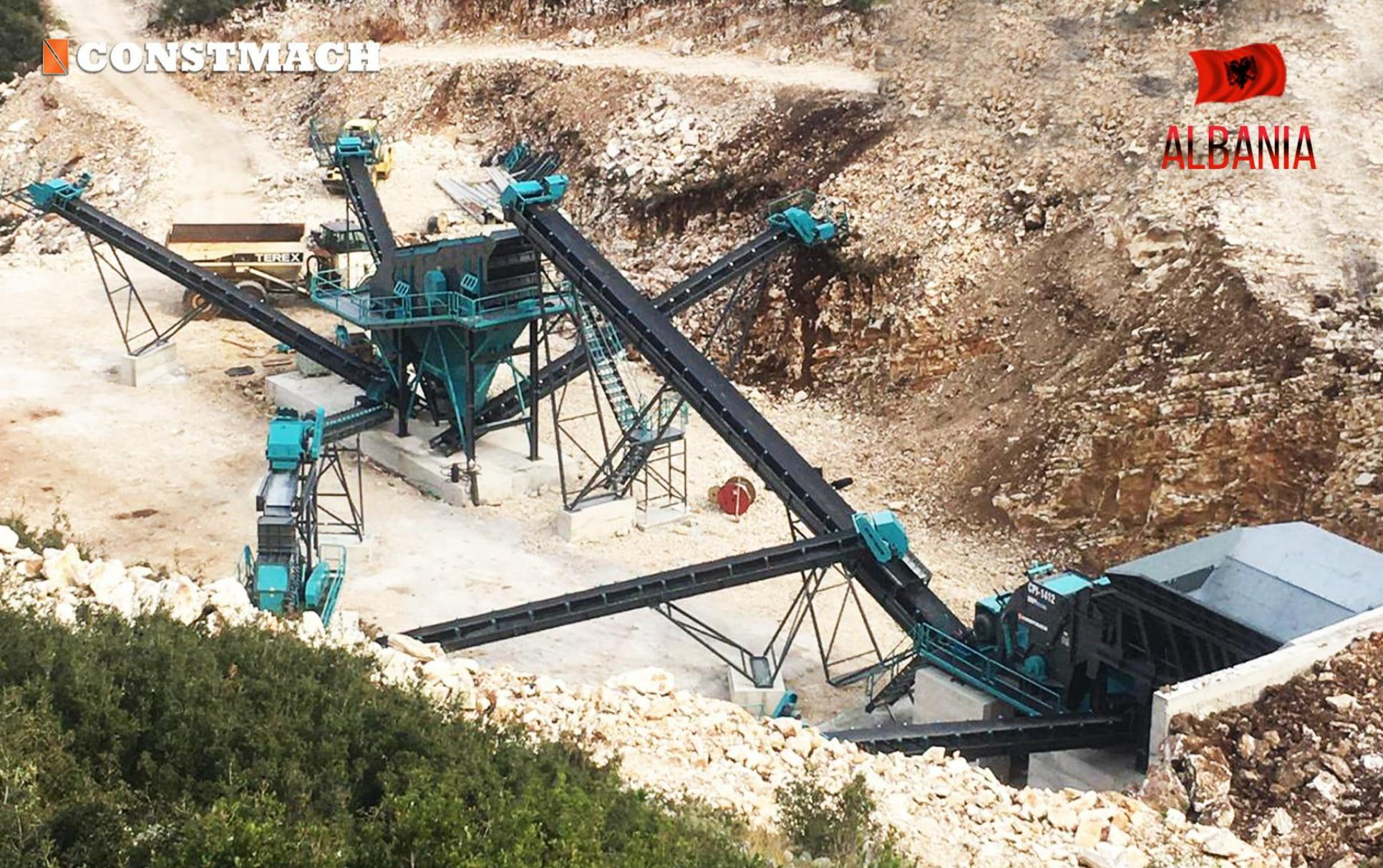
**FIX PI - 2 / STATIONARY CRUSHING AND SCREENING PLANT**
