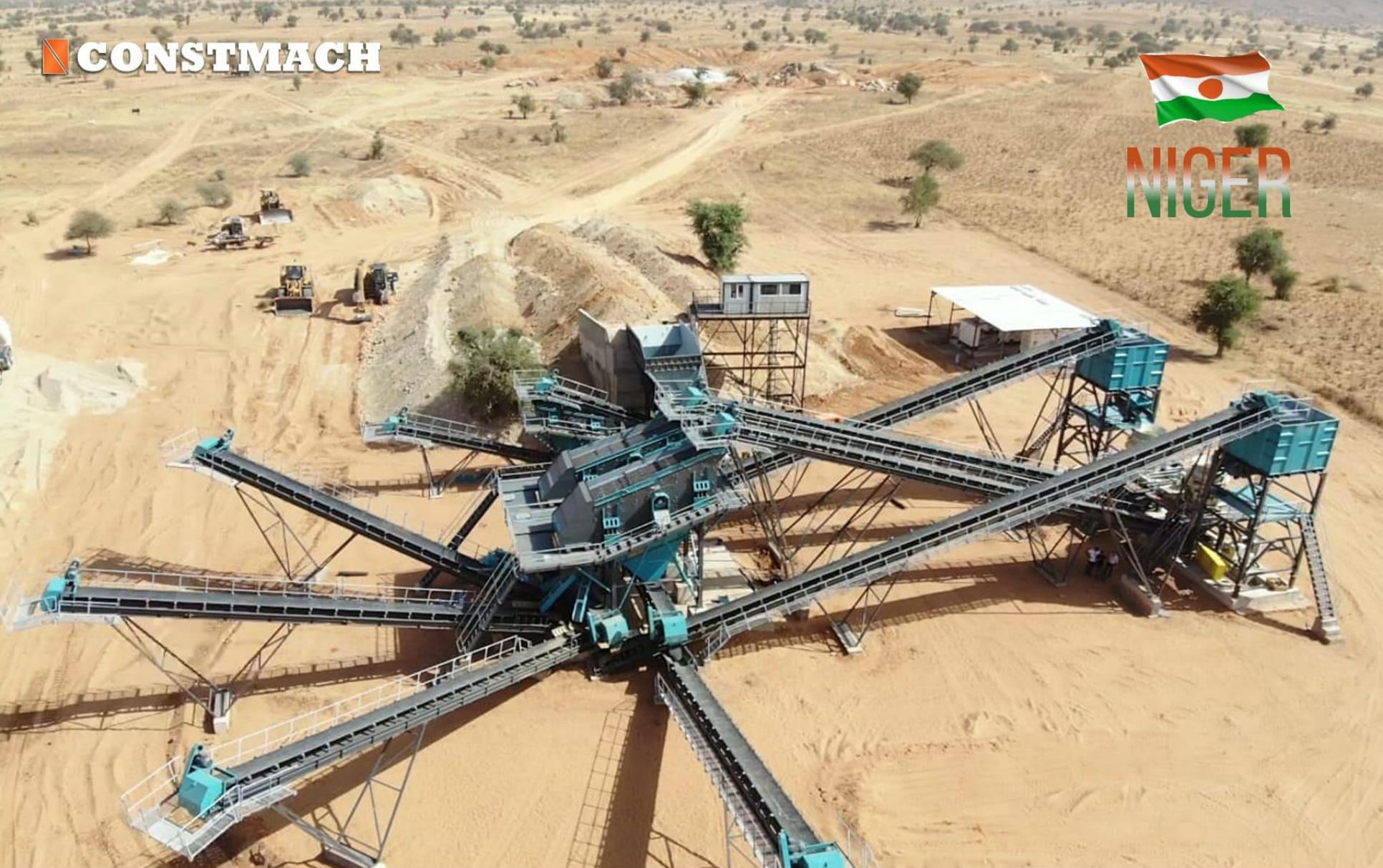
**FIX JCC - 3 / STATIONARY CRUSHING AND SCREENING PLANT**
