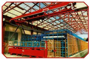
Indoor and OUTdoor solution - travel speed 240 mt/min - lifting speed 30 mt/min - 3 - 4 axis
