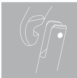
This locking system is recommended in dirty environments, where it's necessary to clean the connector easily.
