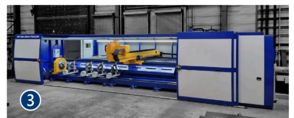
Combined MSF Pro machine for bevel cutting of plates up to 6 x 2 m and pipes up to 6 m length and Ø 300 mm diameter installed in Germany. Pipes and hollow sections are loaded manually from the side through the sliding side panels. The machine has a 6 kW laser source with beam shaping technology.
