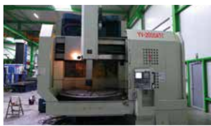
CNC VERTICAL LATHE YOU YI 2500 ATC
