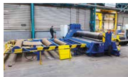
HAEUSLER 4 ROLL PLATE BENDER 3000 MM
