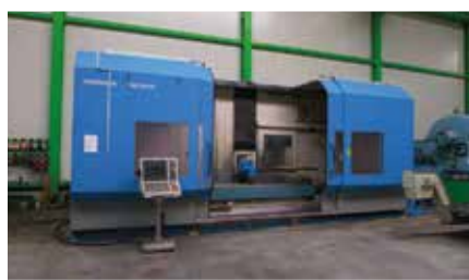
CNC BED MILLING AUERBACH FBE 3000
