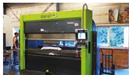
SAFAN E BRAKE PRESSBRAKE 2550 X 65 T
