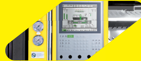
Automatic control Austria made KEBA controller model 2885
