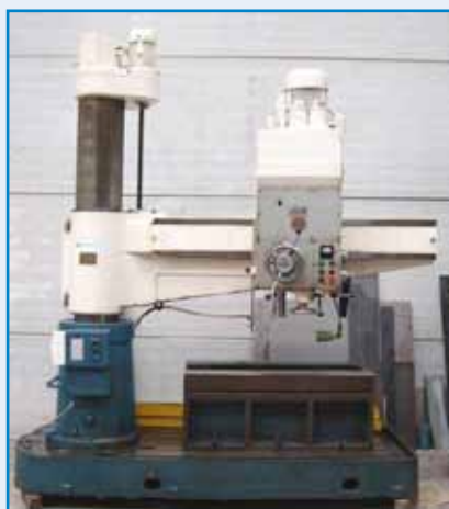
193/I028 STANKO Ø60x1500 mm. • Mesa dado 1.200x600x500mm. 193/I028 STANKO Ø60x1500 mm. • Cube table 1.200x600x500mm.
