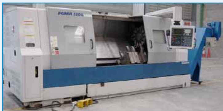
218/P050 Torno DAEWOO PUMA 350 LB. CNC FANUC 0-TF + volante electrónico. E.P. 2000x Ø700 mm. • Palpador • Lunetas • Extractor de virutas. 218/P050 Lathe DAEWOO PUMA 350 LB. CNC FANUC 0-TF + electronic wheel. E.P. 2000x Ø700 mm. • Pre-setter • Steadies • Chip conveyor.
