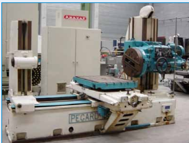
110/J004 PEGARIBERICA . Husillo Ø80 mm. Recorridos 1200x1500x1000 mm. 110/J004 PEGARIBERICA . Spindle Ø80 mm. Travels 1200x1500x1000 mm.
