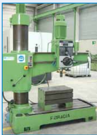
193/N950 FORADIA Ø40x1000 mm. • Mesa dado 650x400x400 mm. 193/N950 FORADIA Ø40x1000 mm. • Cube table 650x400x400 mm.
