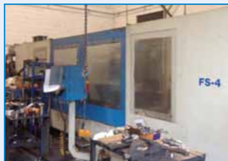
073/Q103 Fresadora bancada fija CME FS-4. CNC FAGOR 8055T. 2007 Recorridos 3000x1200x1000 mm • Refrigeración interna • Carg 24 uds. 073/Q103 Bed type milling machine CME FS4 CNC FAGOR 8055T. 2007 Travels 3000x1200x1000 mm • Internal cooling. • Changer 24 tools.
