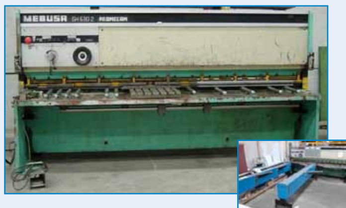
031/M012 MEBUSA GH 630Z . 3000 x 6 mm. Con CNC y tope frontal. 031/M012 MEBUSA GH 630Z . 3000 x 6mm. With CNC and front gauge
