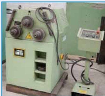
060/P042 Curvadora de Perfiles BPR CPS35 ø35 mm 060/P042 BPR CPS35 Profile Bender machine ø 35mm
