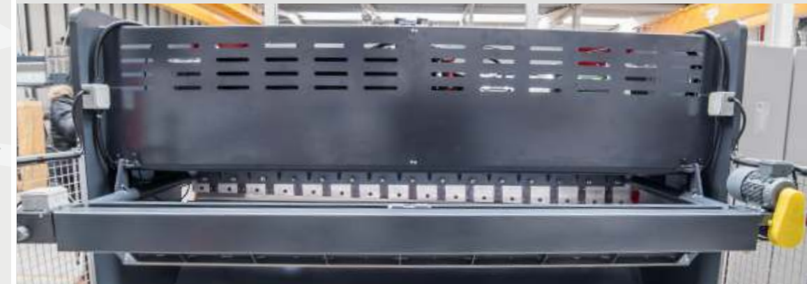
Motorized Back Gauge has \pm 0,1\text{mm} Accuracy
