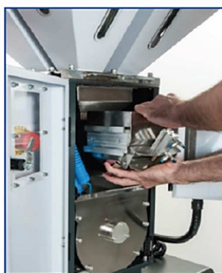
Easy removable weighing chamber
