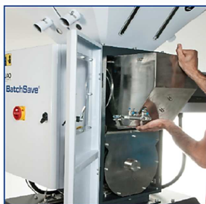
Easy removable weighing chamber
