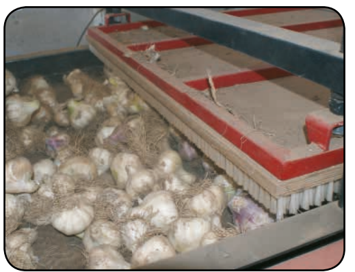
Garlic Brusher Remove the soil, external dry peels and any other parts using rotative brushes without damage the garlic bulbs.
