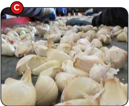
C. Selection and suction belt Two suction areas remove the remains of any bulbs that cannot be used. Any deformed cloves and those without germinating capacity are removed manually from the belt.
