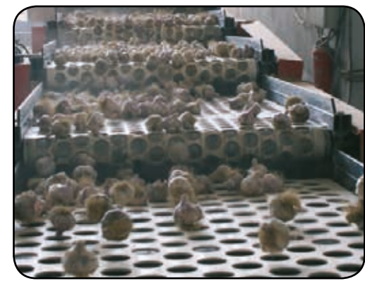
Garlic Grader A consistent size improve the crop profit. The modular grader JJ Broch can be adapted as number of sizes as needed to optimize the crop marketing.
