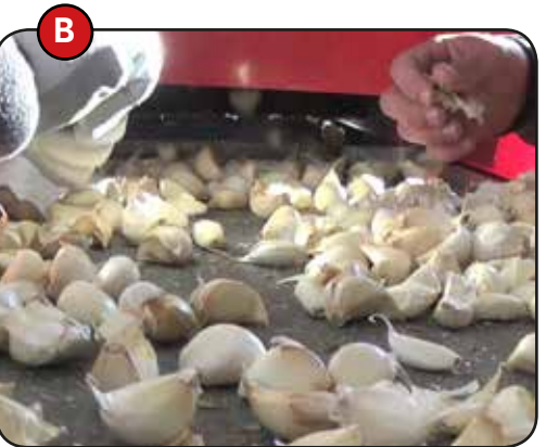
B. Splitter The splitter, equipped with brushes and belts, separates the cloves to prevent pressure and product damage. The position of the belts is adjusted according to the calibre of the cloves.
