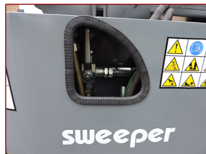
▲ Palanca accionamiento cepillo lateral Hand lever operation side sweeper
