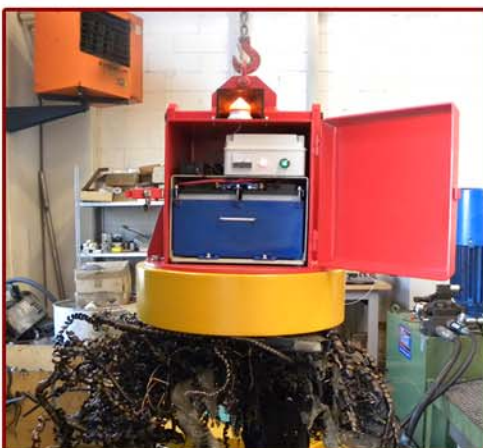
▲ Electroimán activado - magnetizando Electromagnet activated - magnetizing
