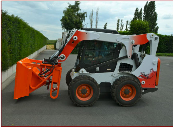
▲ Autocarga del material a esparcir. Self-loading of the material to be spread.
