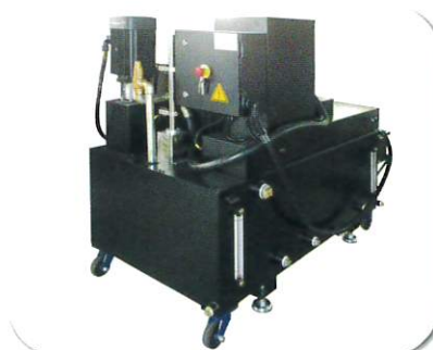
CTS 20 bar separate type with paper filter
