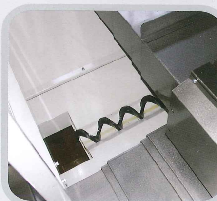
Visinfin extraccion virutas VMC-1600/2100(std)
