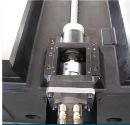
Hollow Ballscrew w/ Oil Cooling System for 3 axes
