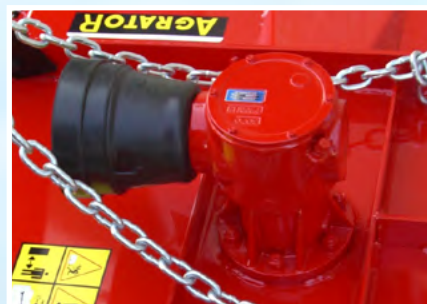
Grupo TdF 540 rpm Boitier PdF 540 tpm Gearbox PTO 540 rpm
