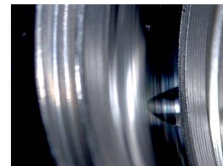
Ball indentation in raceway
