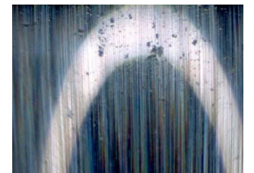
Indentations in raceway caused by particles
