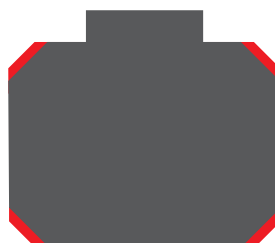
Slitta con quattro guide a V. Slide with four V enlarged shape guides.
