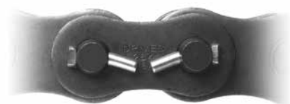
Coated T-pins used on the connecting links.
