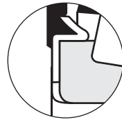
Fig. 1. Backing shoulder against seal backface.
