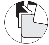
Fig. 2. Backing shoulder against cone (inner-ring) backface (below seal).
