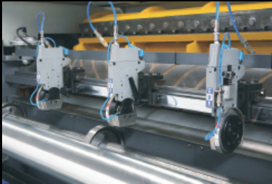
三组分条刀可供修边及对割 Three sets of slitting knife are used for trimming and middle slitting.
