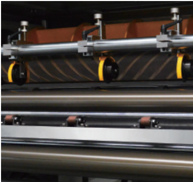
三组分条刀可供修边及对抛 Three sets of slitting knife are used for trimming and middle slitting
