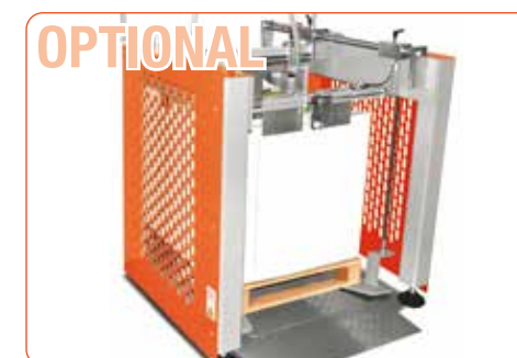
Stacker on delivery: DIGIFAV B2 is available with an optional pallet delivery pile system which can be unloaded using a hand pallet truck or forklift.
