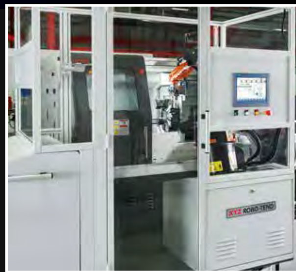
The XYZ ROBO-TEND on an XYZ Turning Centre
