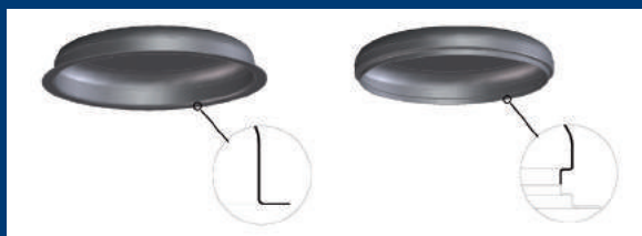
Bordatura e rifilatura coperchi. Beading and trimming of lids.
