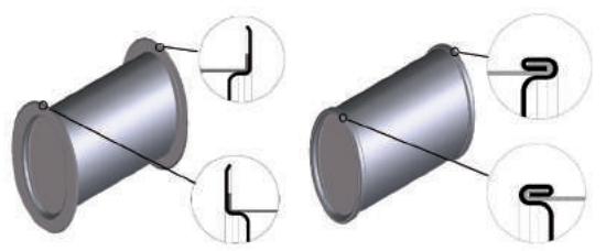
Aggraffatura silenziatori per auto e camion. Lock-seaming of car and truck mufflers.
