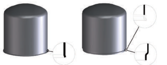
Rifilatura e rifilatura/bordatura interna di semibombole GPL. Trimming and inner trimming/beading of LPG half-cylinders.
