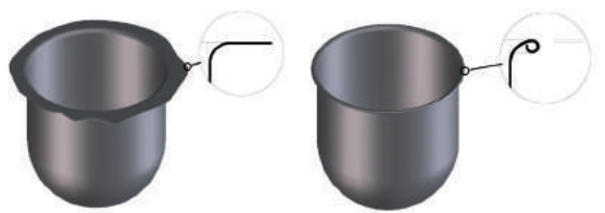
Rifilatura ed arricciatura esterna di vasche inox per macchine impastatrici. Trimming and outer curling of stainless steel tanks for pastry equipment.
