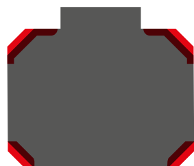
Slitta con quattro guide a V Slide with four V enlarged shape guides
