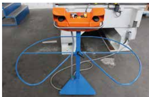
Pulsantiera separata Two-hand control pulpit
