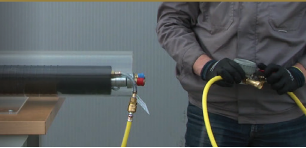
Water test according to EN 1610
