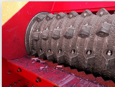
Rotating and Interchangeable Blades – Heat treated Blades Holders
