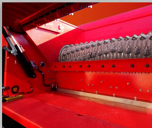
Rotor back door with bolts-free hydraulic opening.
