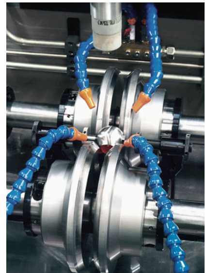
Workpieces of only 8mm diameter can also be machined.
