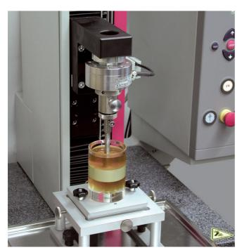
Fig. 1: Zwick Roell back extrusion rig
