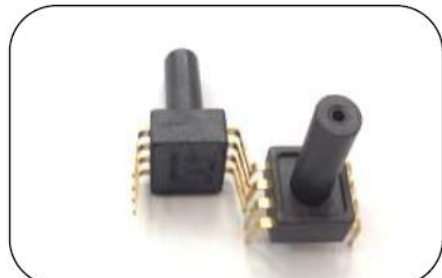
Water Level Sensor
