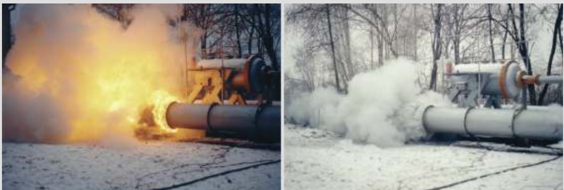
Test photos: Dust explosion in a pipe without and with RSBP HRD barrier
