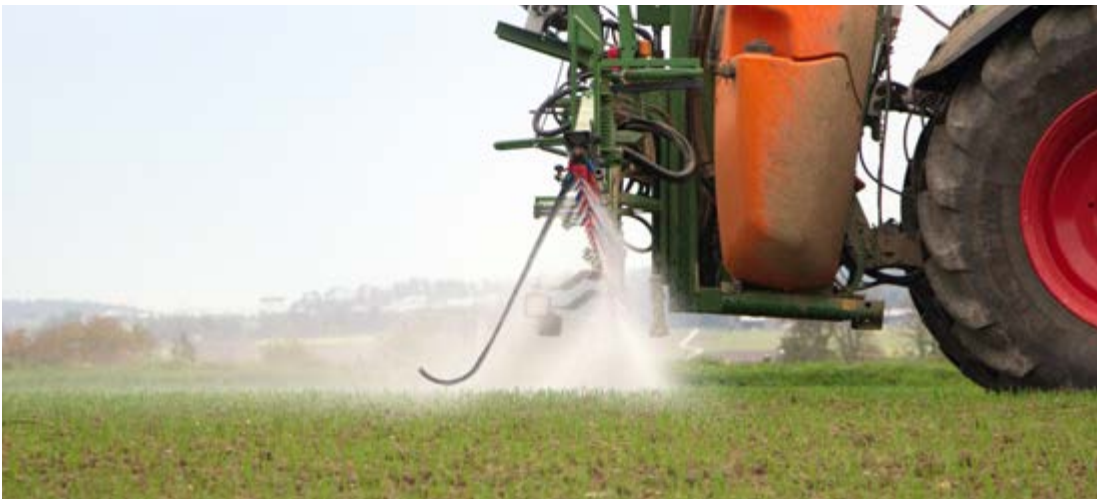
Optimal coverage through the twin flat spray nozzle
