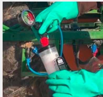
Calibrating twin flat spray nozzles with SPOTON
