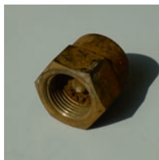
Clogged vane of a full cone nozzle
