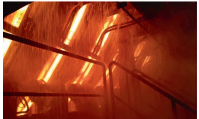
Secondary cooling zone of billet caster
